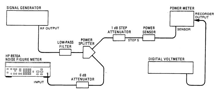
Figure 4-2. Noise Figure Instrumentation Accuracy Test Setup
