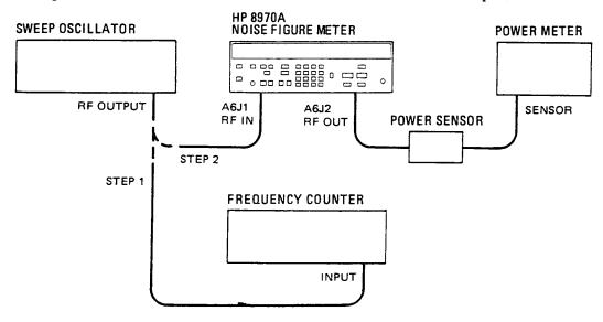
Figure 5-9. 20 dB Input Amplifier Gain Adjustment Setup
