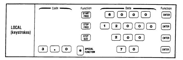
e. To calibrate the Noise Figure Meter, set up the equipment as shown below.
