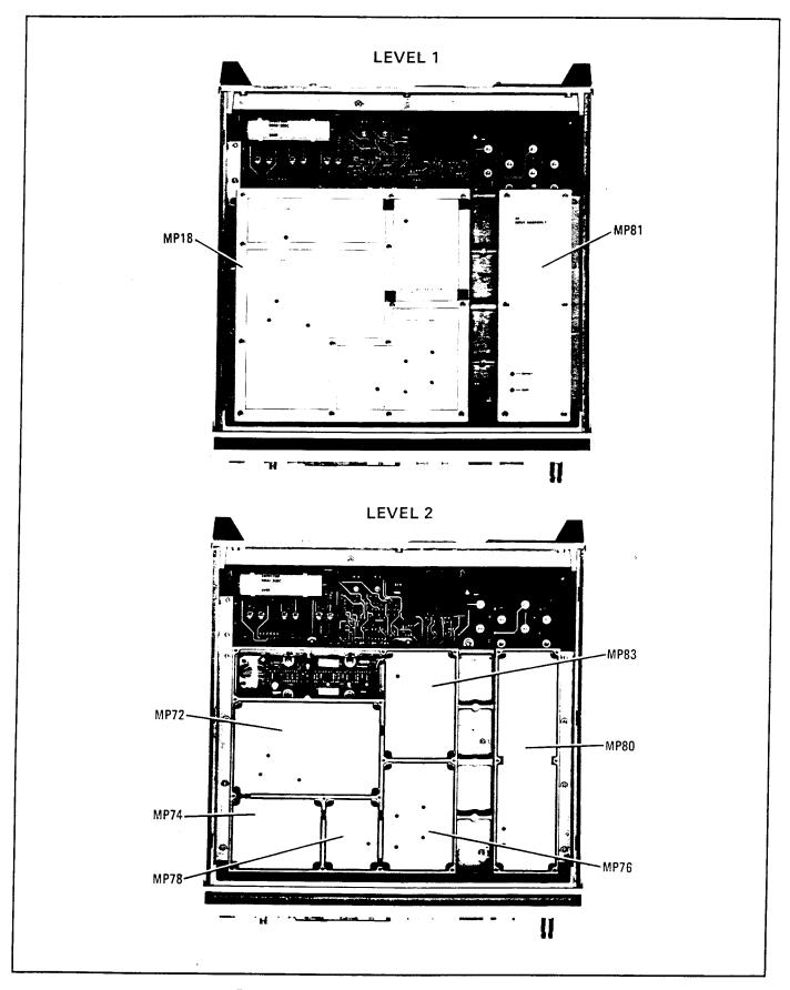
Figure 6-5. Top Internal RF Covers Identification
