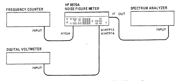
Figure 5-7. Frequency Cal RF Detector and First LO Offset Adjustment Setup
