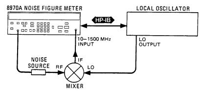
f. Calibrate the equipment in Measurement Mode 1.1 by pressing CALIBRATE.
