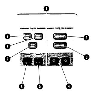
1 Frequency Function Keys. In addition to the functions described below, the following keys are used to prefix numeric entries for the specified functions: START FREQ, STOP FREQ, STEP SIZE, FREQ, and FREQ INCR. Frequency is entered in MHz from the front panel. Frequency parameters are entered in a Function — Data — ENTER format.
