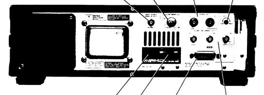
Line Power Module permits operation from 100, 120, 220 or 240 Vac. The number visible in the window indicates nominal line voltage to which the instrument must be connected (see Figure 2-1). Center conductor is a chassis connection for safety earth ground.
