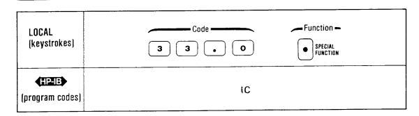
Program Codes The HP-IB code for IF Attenuator Calibration is IC (or 33.0SP).
