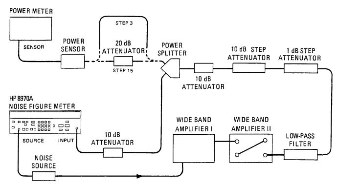
Figure 4-3. Gain Measurement Uncertainty Test Setup
