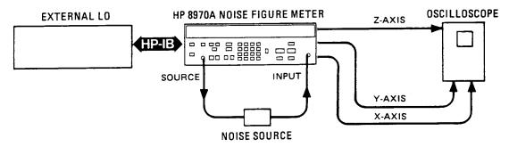
Figure 3-8. Basic Functional Checks Setup
