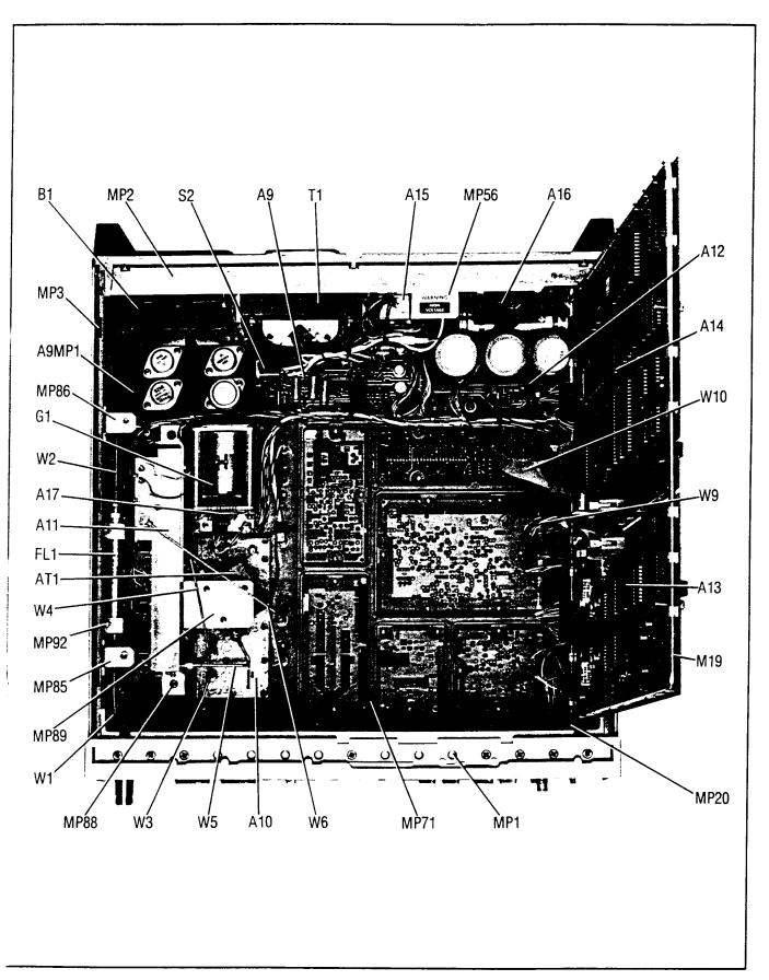
Figure 6-4. Bottom Chassis Parts, Mechanical Parts, and Cable Identification
