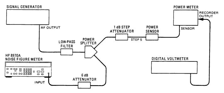
Figure 5-1. Noise Power Detector Adjustment Setup
