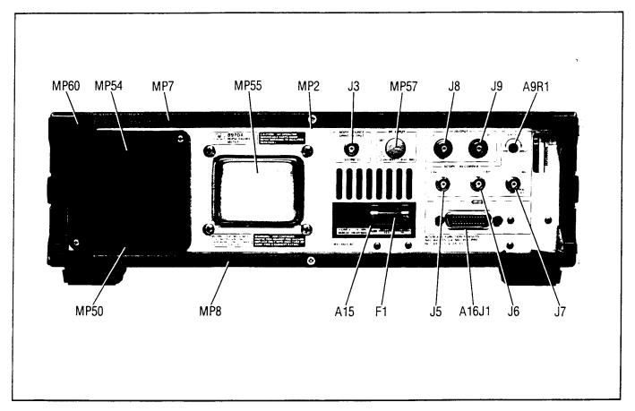
Figure 6-2. Chassis and Mechanical Parts Identification — Rear Panel
