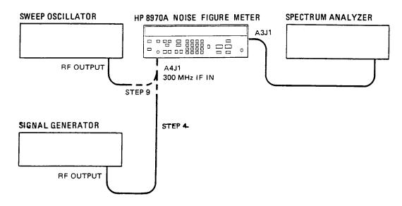
Figure 5-3. 300 MHz IF Bandpass Filter Adjustment Setup
