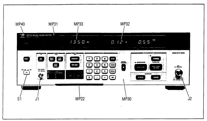
Figure 6-1. Chassis and Mechanical Parts Identification — Front Panel
