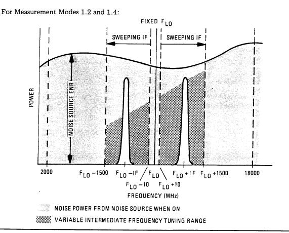
Noise Figure Meter Measurement Passband
