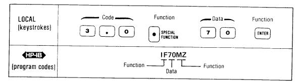
Program Codes The HP-IB codes for Hz and MHz are HZ and MZ, respectively. For Special Function 3 program codes, refer to Procedure.
