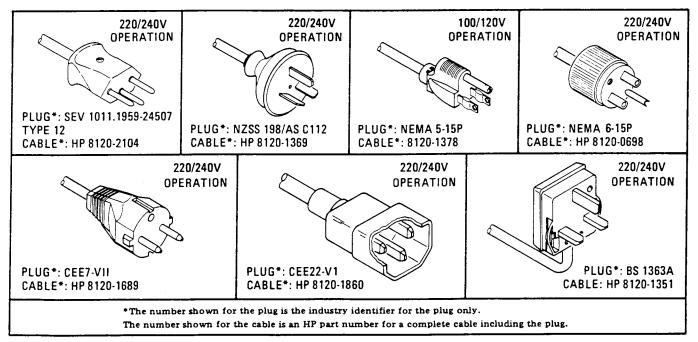
Figure 2-2. Power Cable and Mains Plug Part Numbers
