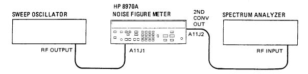
Figure 5-6. 2050 MHz Bandpass Filter Adjustment Setup
