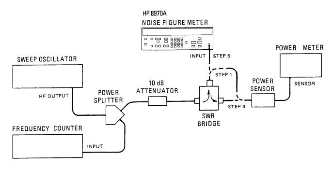
Figure 4-1. Input SWR Test Setup
