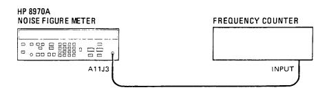
Figure 5-5. Second Converter LO Frequency Adjustment Setup
